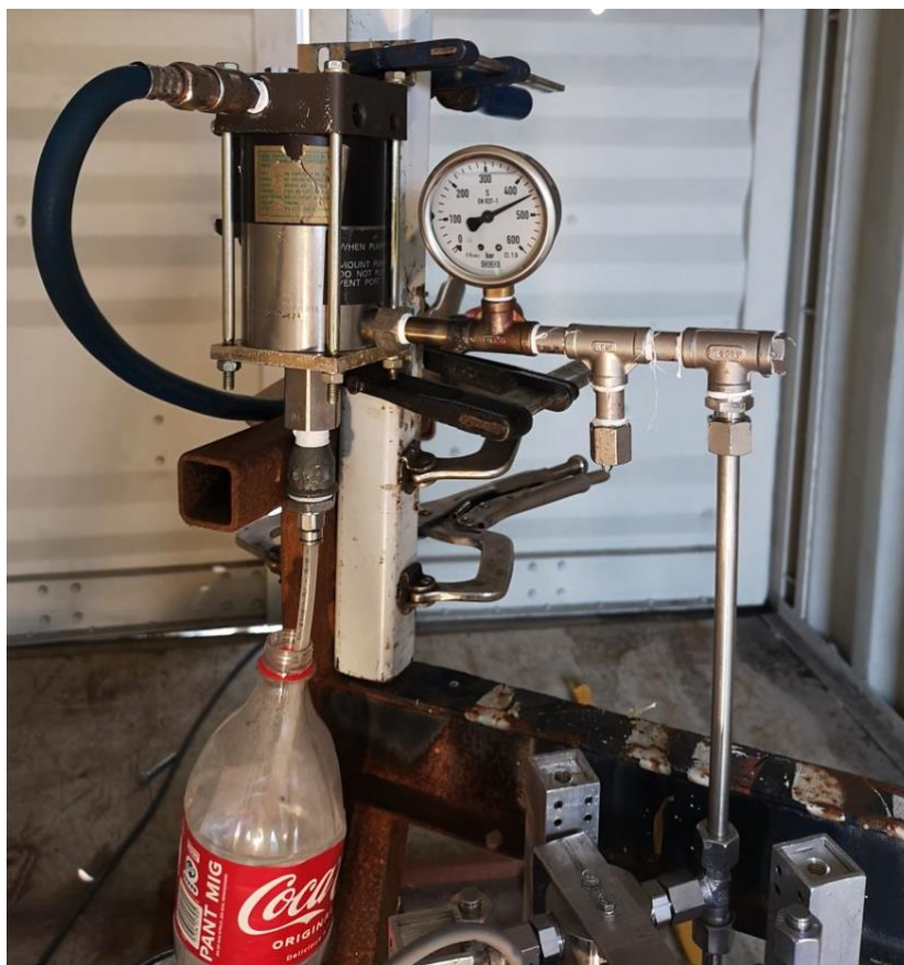
Figure 12: “Maximator” testing a Dynamic Pressure Regulation system for a bi-liquid, checking for leaks. (Source: Copenhagen Suborbitals)
