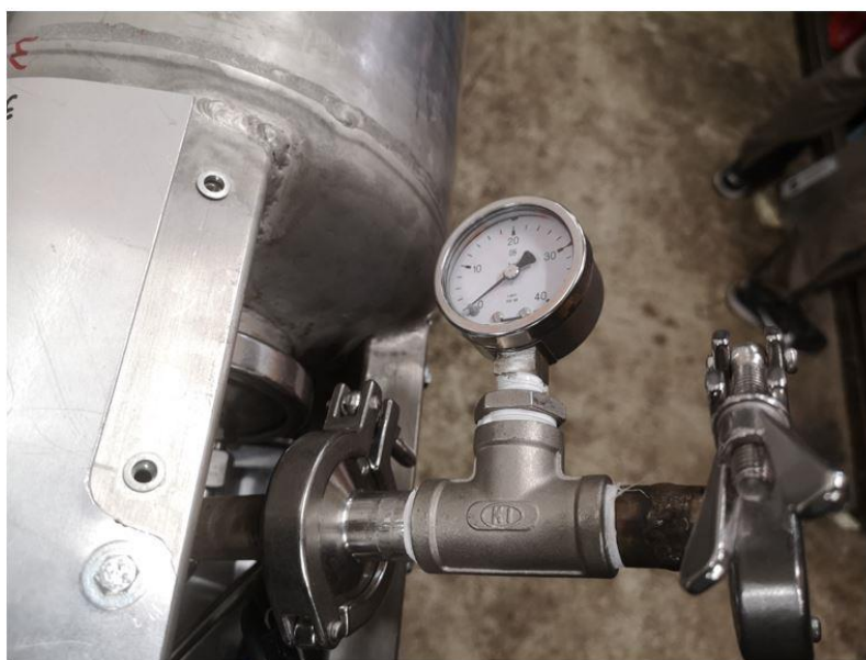
Figure 11: A handy burst disc "extender" for AIT purposes. (Source: Copenhagen Suborbitals)
