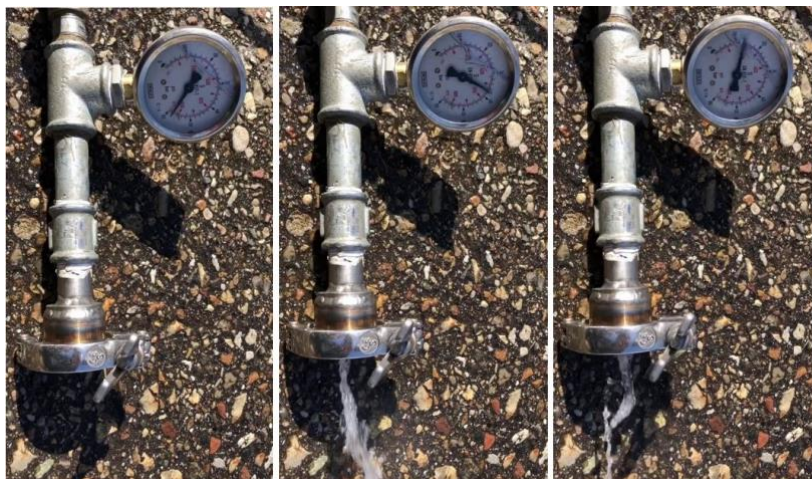
Figure 8: Frame grabs from a rupturing burst disc. (Source: Copenhagen Suborbitals)
