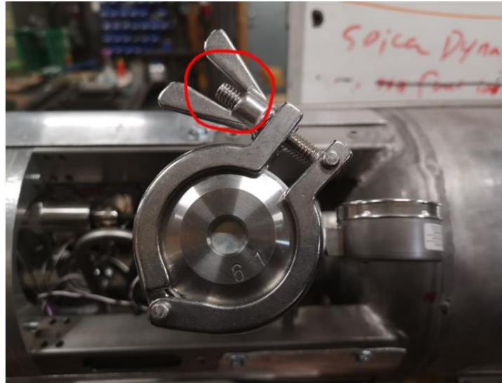
Figure 9: Nominal clamp position with one burst disc. (Source: Copenhagen Suborbitals)
