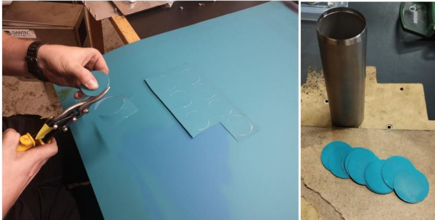
Figure 4: Initial burst discs cut by hand. Simple punching tool allowing “mass production” of discs. (Source: Copenhagen Suborbitals)
