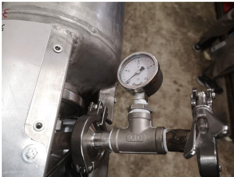
Figure 11: A handy burst disc "extender" for AIT purposes. (Source: Copenhagen Suborbitals)
