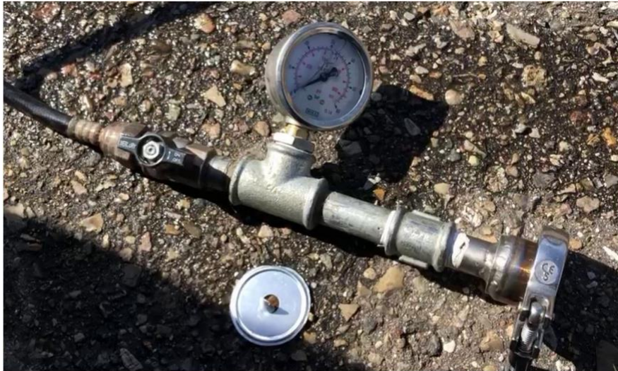
Figure 6: A simple burst disc test rig and an example of a ruptured burst disc. (Source: Copenhagen Suborbitals)
