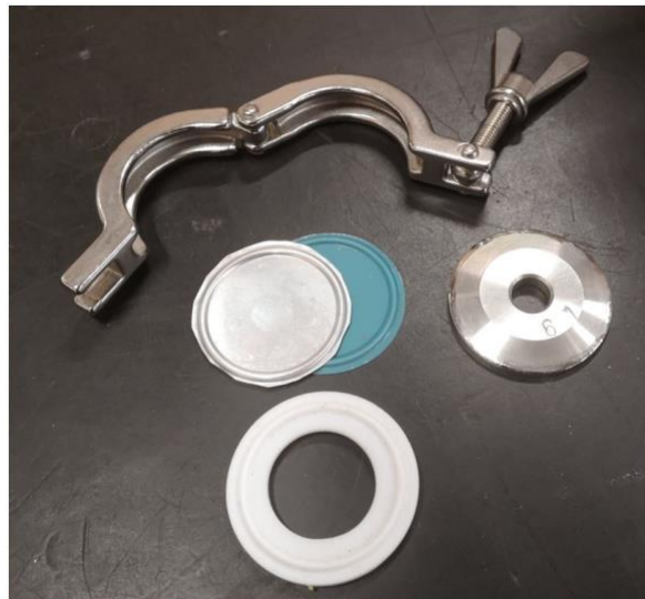
Figure 5: An early SRAD burst disc “set” based on COTS clamp ferrule parts. (Source: Copenhagen Suborbitals)
