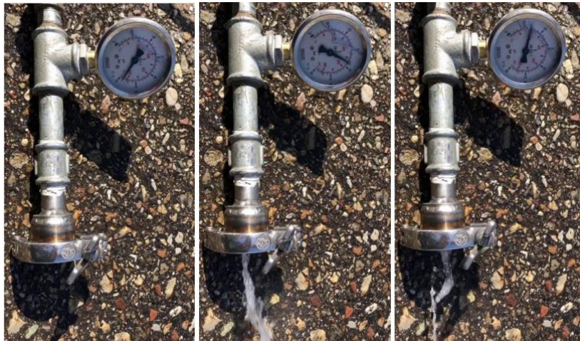
Figure 13: Frame grabs from a rupturing burst disc. (Source: Copenhagen Suborbitals)
