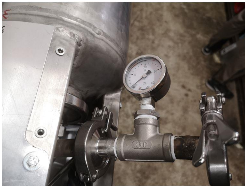
Figure 16: A handy burst disc "extender" for AIT purposes. (Source: Copenhagen Suborbitals)
