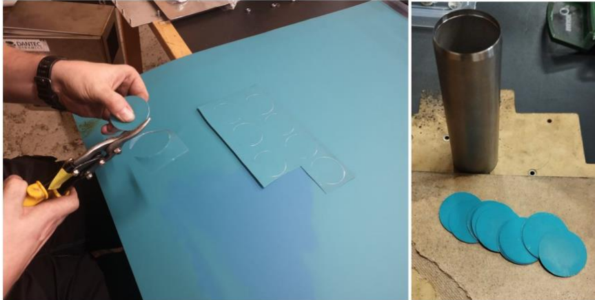
Figure 9: Initial burst discs cut by hand. Simple punching tool allowing “mass production” of discs. (Source: Copenhagen Suborbitals)
