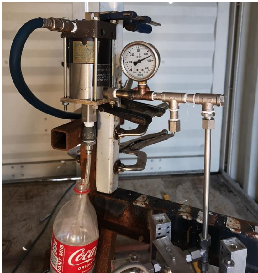
Figure 17: “Maximator” testing a Dynamic Pressure Regulation system for a bi-liquid, checking for leaks. (Source: Copenhagen Suborbitals)
