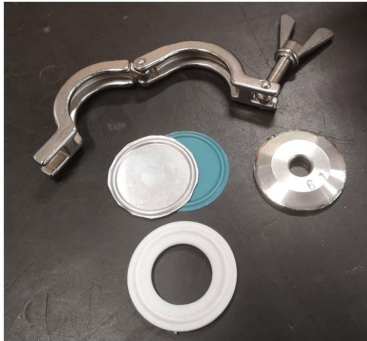
Figure 10: An early SRAD burst disc "set" based on COTS clamp ferrule parts. (Source: Copenhagen Suborbitals)
