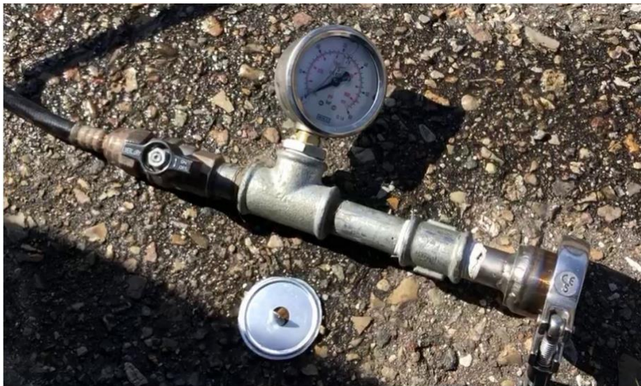
Figure 11: A simple burst disc test rig and an example of a ruptured burst disc. (Source: Copenhagen Suborbitals)
