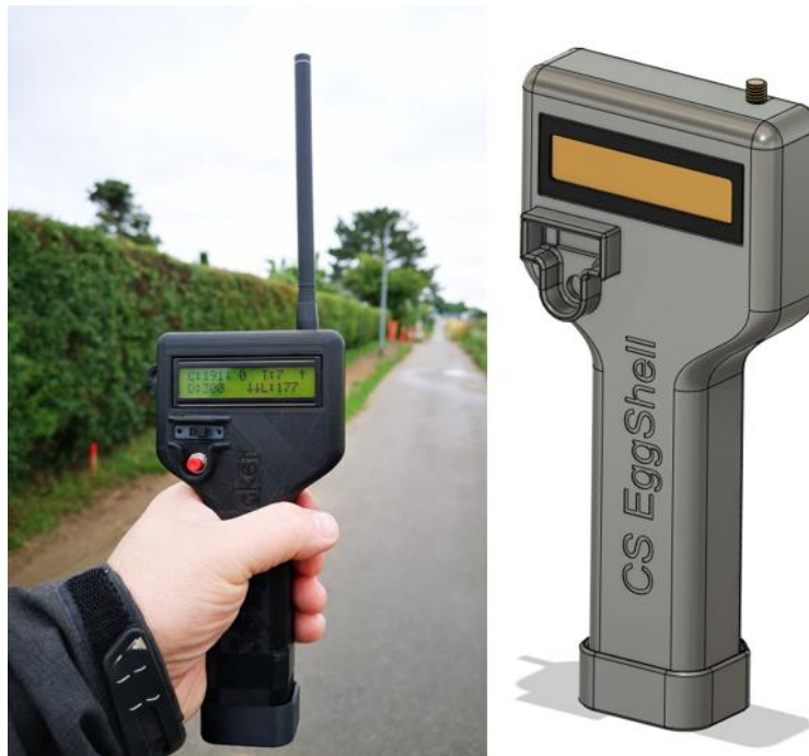
Figure 15: Updated ruggedized custom enclosure for the LCD handheld receiver. (Source: Jacob Larsen)
